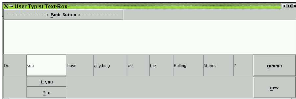
Figure 4.4: Screenshot from the keyboard input module. The screen shows the spelling correction phase after typing is complete. Simple keyboard commands allow the selection of spelling variants found in the dictionary.
